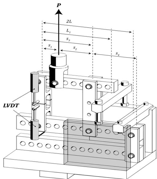
Figure 2 – Apparatus used for the mixed-mode loading conditions [1].
