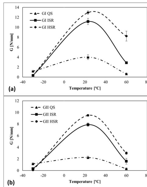
Figure 5 – Fracture energy as a function of temperature: (a) Mode I part (b) Mode II part.
