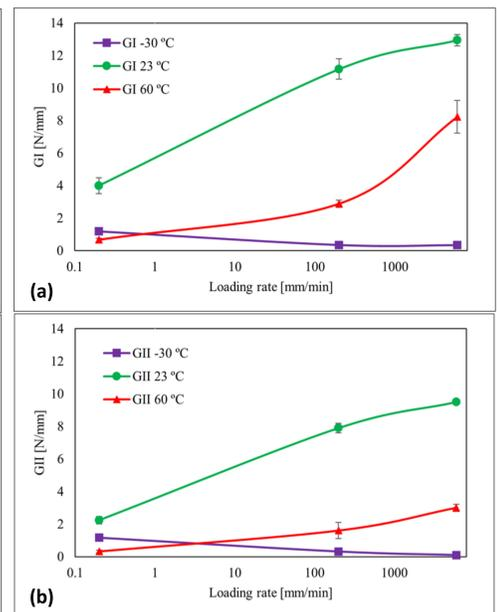
Figure 6 – Fracture energy as a function of loading rate: (a) Mode I part (b) Mode II part.
