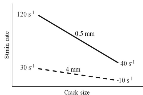
Figure 7 – True strain rate as a function of crack size for both adhesive thicknesses.
