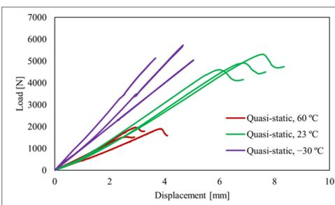
Figure 3 – Load-displacement of the machine for test submitted to quasi-static conditions for a mixed mode apparatus set up at  $45^{\circ}$ .
